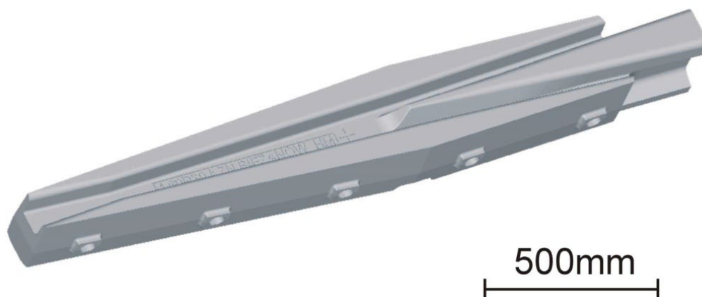
Fig. 1. Scheme of Insert frog R500 (R – turnout radius in meters)
