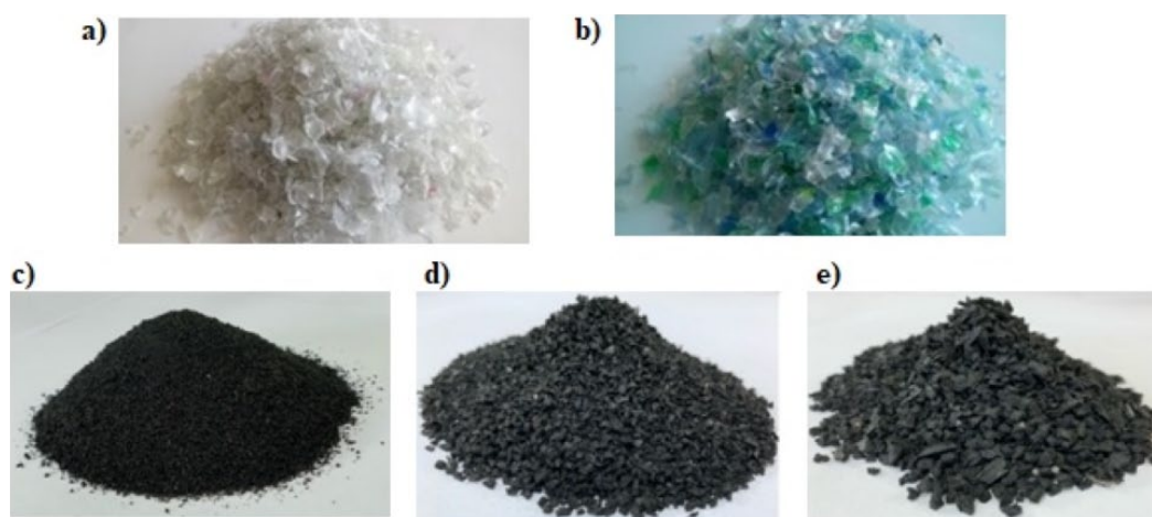
Fig. 1. Waste obtained from recycling: a) colorless PET flakes, b) colored PET flakes, c) SBR rubber granulate, fraction 0\div1 mm, d) SBR rubber granulate, fraction 0.8\div2 mm, e) SBR rubber granulate, fraction 2\div4 mm
