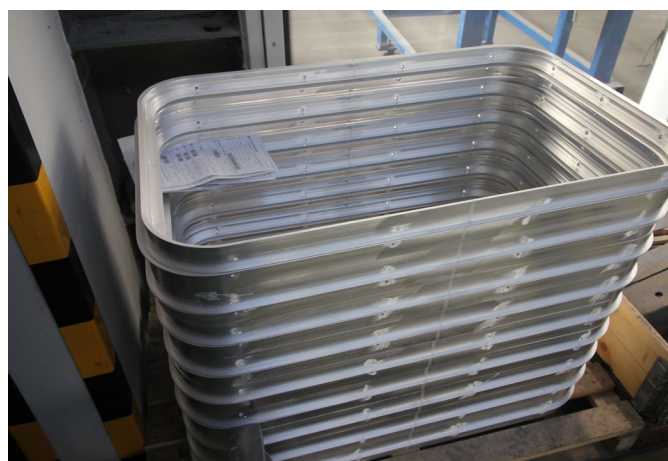
Fig. 2. The window frame is made of tested aluminium alloy
