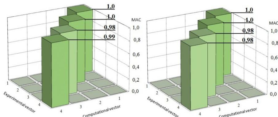
Fig. 7. Histogram of MAC values – direction y: a) MB model, b) MS model
