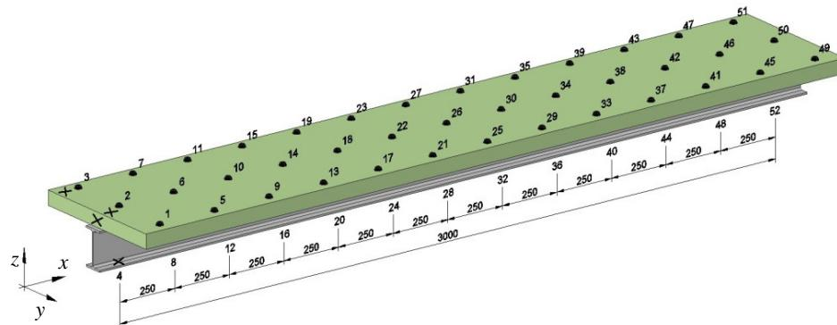
Fig. 2. Grid of measurement points
