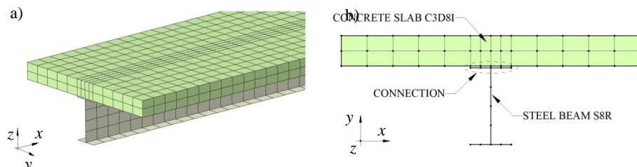
Fig. 3. FEM model of the analysed composite beam: a) a view of the beam, b) cross-section
