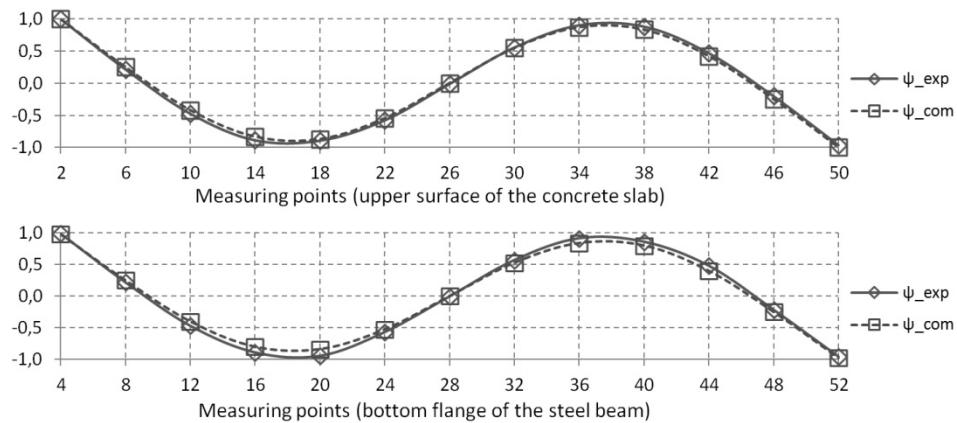
Fig. 6. Comparison of normalized modal vectors, second mode of flexural vibrations
