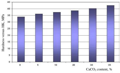
Fig. 3. Hardness versus CaCO<sub>3</sub> content
