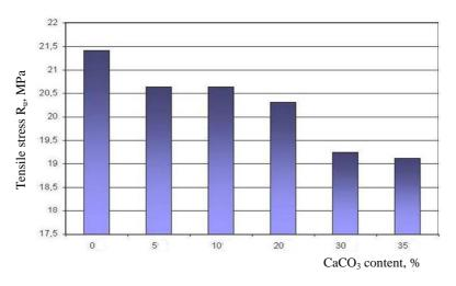
Fig. 1. Maximum tensile stress  $R_u$  versus CaCO<sub>3</sub> content
