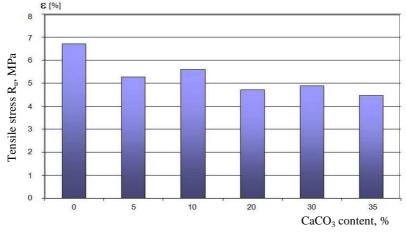
Fig. 2. Elongation at R<sub>u</sub> versus CaCO<sub>3</sub> content
