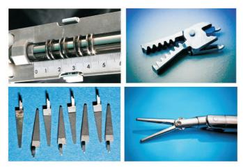
Fig. 2. NCD covered and ceramic elements of tools
