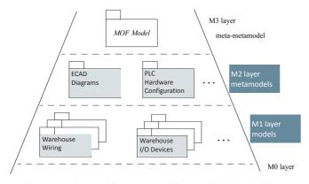
Fig. 5. Metadata architecture according to ISO/IEC 19502 [7]
