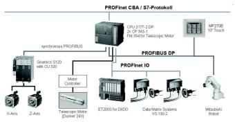
Fig. 2. Example of the automation structure of a storage and retrieval
