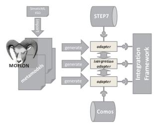
Fig. 7. Complete TiE architecture for tool-integration
