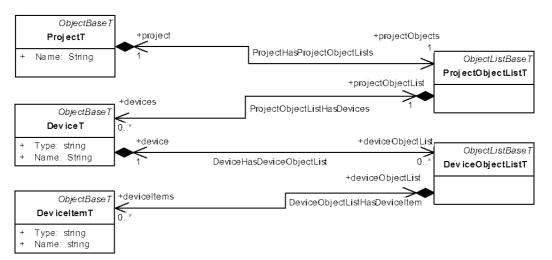
Fig. 9. Excerpt from SimaticML metamodel
