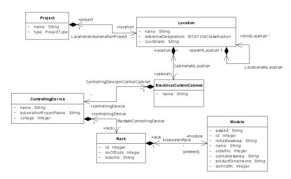
Fig. 8. Location-oriented model metamodel in correspondence to IEC 61346 (Ref. 15)
