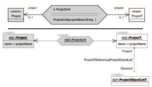
Fig. 10. ProjectLink definition and appropriate TGG rule
