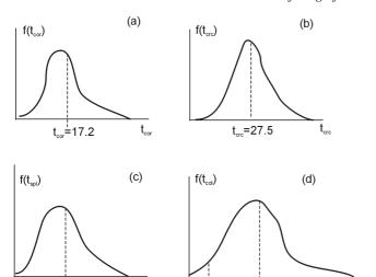
Fig. 4. Probability density functions of random variables  $t_i$  (years): (a) corrosion initiation time  $t_{cor}$ , (b) cracking initiation time  $t_{crc}$ , (c) spalling initiation time  $t_{spl}$ , (d) time to collapse  $t_{col}$
