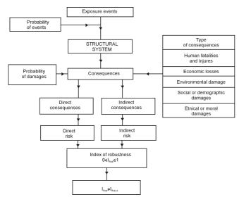
Fig. 1. Stages of the structural robustness assessment according to the probabilistic risk-based approach
