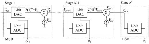
Fig. 15. Block diagram of a Gray algorithmic ADC
