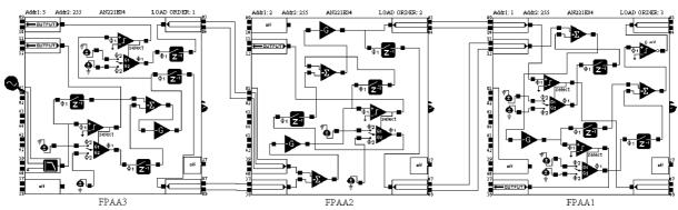
Fig. 10. Circuit realization of a 6-bit serial algorithmic ADC
