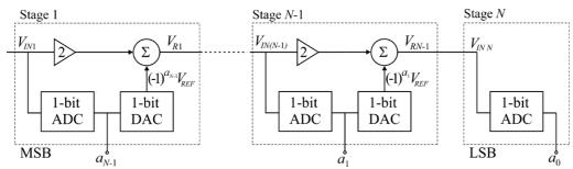
Fig. 9. Block diagram of a serial algorithmic ADC
