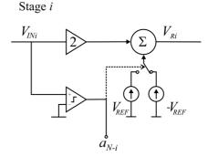
Fig. 8. Structure of i-th stage of the serial ADC
