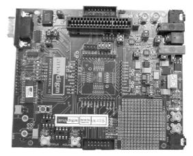
Fig. 1. Anadigm Vortex AN220D04 Evaluation Board whit the AN221E04 device
