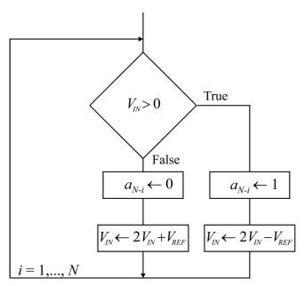
Fig. 2. Flow chart of an iterative algorithmic ADC
