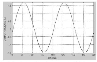
Fig. 19. Sinusoidal waveform after reconstruction digital outputs of the Gray algorithmic 6-bit ADC
