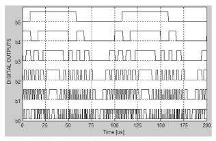
Fig. 12. Digital outputs of the serial algorithmic 6-bit ADC
