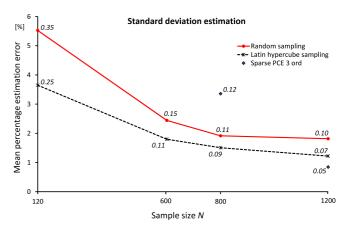
Fig. 4. The turbo-generator rotor shaft example. Mean relative percentage error of the standard deviation estimation of the maximal rotor-shaft vibration amplitude obtained using RS, LHS and sparse
