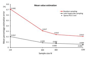
Fig. 3. The turbo-generator rotor shaft example. Mean relative percentage error of the mean value estimation of the maximal rotor-shaft vibration amplitude obtained using RS, LHS and sparse PCE
