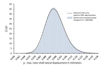
Fig. 2. The maximal lateral displacement histogram obtained with random sampling (sample size  $N=1\,000\,000$ ) and the corresponding MEP-based PDF
