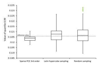
Fig. 9. Box plots for MEP-based 0.99 quantile computation for various methods of statistical moments estimation (sample size N=1200). The reference value is established by an extensive  $(N=1\,000\,000)$  random sampling
