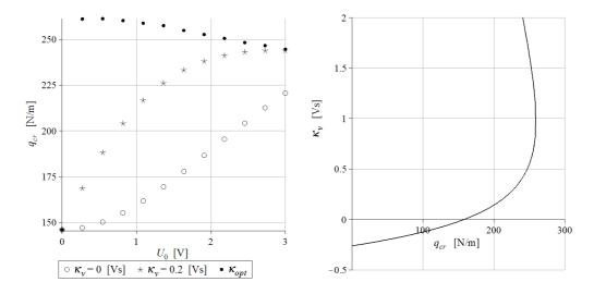
Figure 3. Critical compressive load for the control depending on velocity and without active control (on the left) and the relation between this load and the control for  $U_0 = 1 \text{ V (right)}$ ,  $x_e = 0.33L$ , air.
