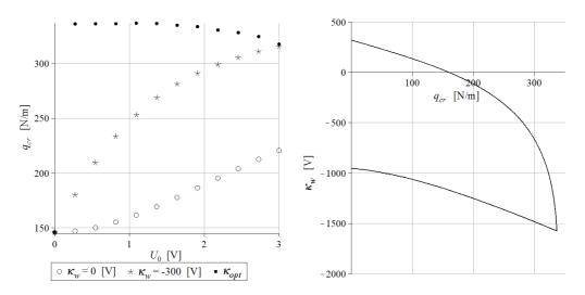
Figure 2. Critical compressive load for the control depending on the displacement and without the active control (on the left) and the relation between this load and the control for  $U_0 = 1$  V (right),  $x_e = 0.33L$ , air.
