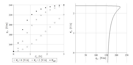
Figure 4. Critical compressive load for the simple control depending on the current and without active control (on the left) and the relation between this load and the control for  $U_0 = 1 \text{ V}$  (right),  $x_e = 0.33L$ , air.
