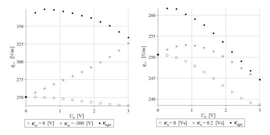
Figure 5. Critical compressive load for control depending on the transverse displacement (on the left) and on the velocity (right),  $x_e = 0.33L$ , water.
