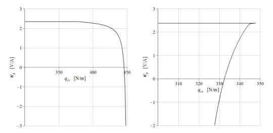
Figure 9. Relation between the critical tension and the simple control depending on the current for  $U_0 = 0.5$ V (on the left) and  $U_0 = 3$  V (right),  $x_e = 0.33L$ , air.
