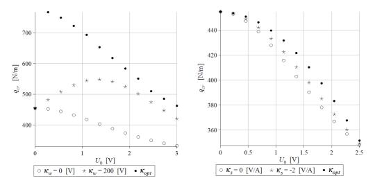
Figure 10. Critical tensional load for the control depending on the displacement (on the left) and on the current (simple one, right),  $x_e = 0.33L$ , air.
