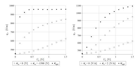
Figure 6. Critical tensional load for control depending on the transverse displacement (on the left) and on the current (right),  $x_e = 0.50L$ , air.
