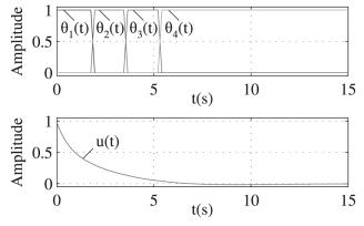
Figure 2: Calculated switching parameters  $\theta(t)$  and the controller output with switched controller (22) – QS
