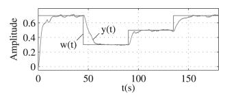
Figure 5: Measured results w(t), y(t) with switched controller (25)
