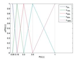
Figure 6. Membership functions used in Takagi-Sugeno fuzzy logic interface module.
