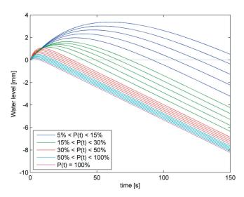
Fig. 4. Family of unit step responses  $Q_{\nu}$  of the steam generator models.
