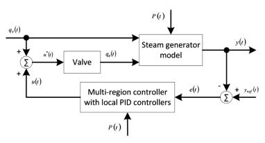
Fig. 1. Steam generator water level control structure.
