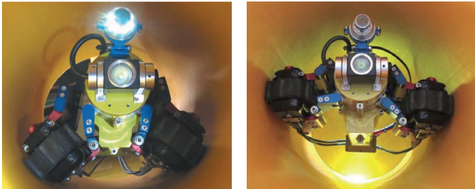
Fig. 5. Operation environments: a) horizontal pipe, \varnothing 235 mm , b) vertical pipe, \varnothing 235 mm
