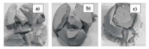
Fig. 2. Photo of solidified spent drilling mud sample using 4% sodium silicate and 25% Silment CQ 25 a) bentonite drilling mud, b) potassium-polymer drilling mud, c) glycol-potassium-polymer drilling mud
