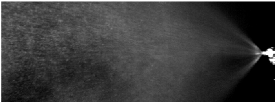
Fig. 6. Generating of droplets by the swirl jet with use of water flow 0.6 l/min and pressure of 0.45 MPa
