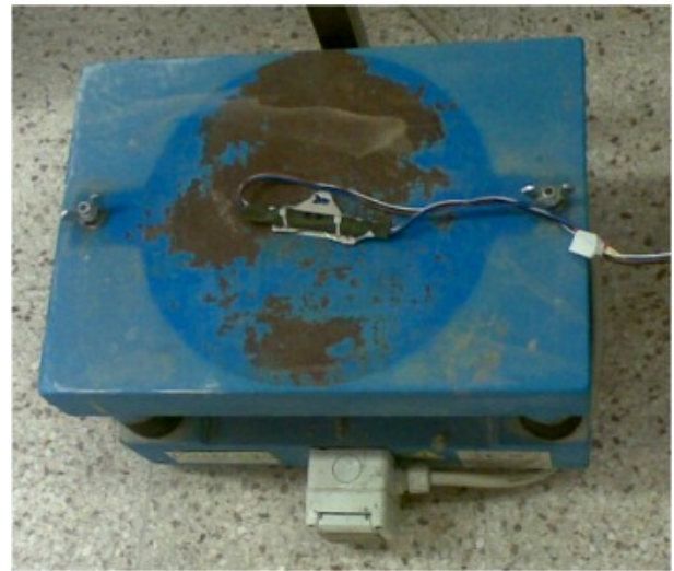
Fig. 15. Vibrating table with attached accelerometer.
