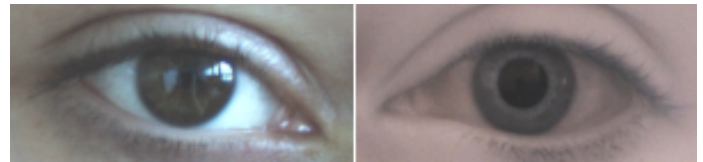
Fig. 2. Example images of the same eye done with the non-modified camera done in the visible range of light (left) and done with the same modified camera in near-infrared spectrum (cutoff light length 715nm) (right).
