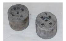
Fig. 7. Ready briquettes containing post-reclamation dust bonded with cement binder
