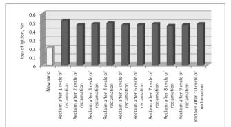
Fig. 2. Loss on ignition in materials from the multiple reclamation of self-hardening sands
