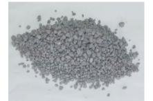
Fig.8. A sample of the granulated post-reclamation dust
