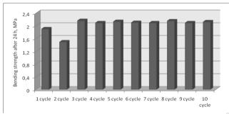
Fig. 4. Bending strength of sands with reclaim from multiple reclamation
