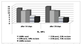
Fig. 5. The results of compression test carried out on samples of concrete with the variable content of reclaim
