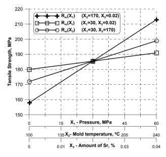
Fig. 1. The influence of squeeze pressure, mould temperature, and quantity of modifier on the tensile strength of castings made of AlSi7Mg alloy
