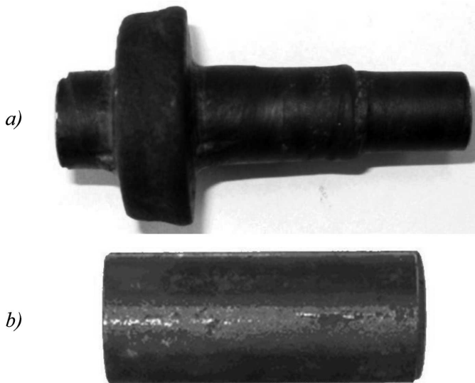
Fig. 13. Shape of part formed in CWR with upsetting (extreme allowances removed) – a, billet used in rolling – b
