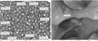
Fig. 4. The specified thickness of selected branch of foam filter A and the remains of the polyurethane skeleton
