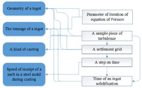
Fig. 3. Diagram of influence of parameters
