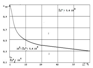
Fig. 2. Diagram of a mathematical model selection depending on the effective size and overheating: 1 – non convective model, 2 – laminar convection, 3 – turbulent convection
