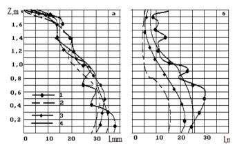
Fig. 1.. Solid skin thickness against height of 15.3 ton ingot with bottom casting (a) and top casting (δ); curve 1 shows the experimental results, curve 2 represents calculation without turbulence considered, curve 3 – with regard to turbulence, curve 4 – with regard to turbulence and a gas phase
