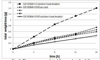
Fig. 8. The wear curves plotted for samples after full abrasion cycle, [14]
