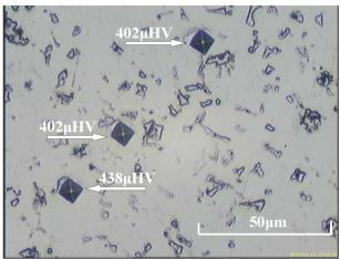
Fig. 7. Cast steel microstructure after solution heat treatment; nital etched;
