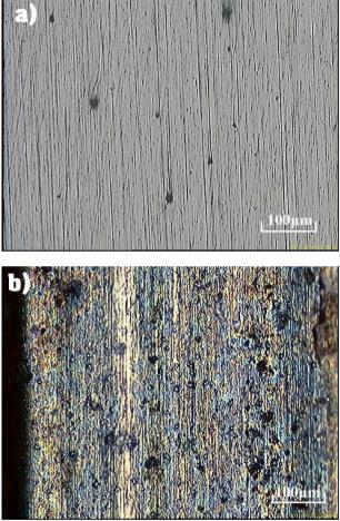
Fig. 9. Surfaces of samples after abrasion test, (a) – cast Hadfield steel after solution heat treatment, (b) - cast steel with carbides
