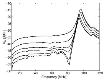
Fig. 4. H(f) versus distance d = D, 1.25D, 1.5D, 1.75D, 2D, 2.5D, with the coil diameter D = 4 cm
