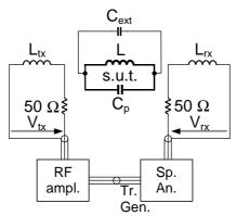
Fig. 2. Measurement setup with coupled transmitter and receiver coils and interposed s.u.t.
