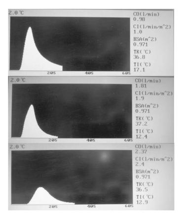
Fig. 7. Screenshots of the patient's monitor -CO measurements by be means of thermodilution carried out on physical model of the pulmonary circulation.
