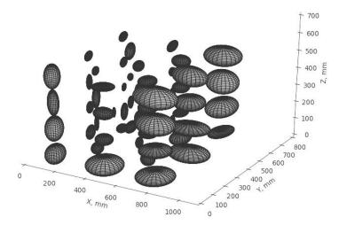
Fig. 5. Values of residual errors presented as ellipsoids of the point reproduction error.
