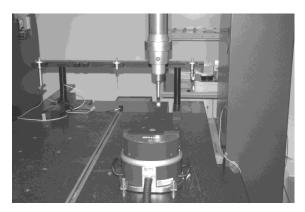
Fig. 1. Cooperation between the CMM and LaserTracer.
