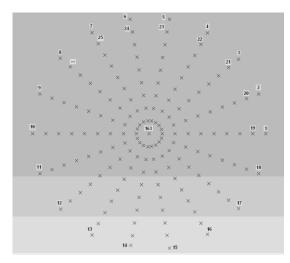
Fig. 4. Measuring sequence, points indicated by "x" are nods of reference grid (view from top of the test sphere).
