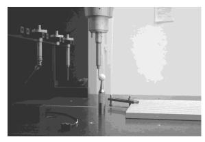
Fig. 3. Measurements of test sphere performed on Leitz PMM 12106 machine equipped with a Leitz measuring probe head.
