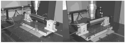
Fig. 7. Measurements of a standard cylinder.
