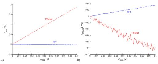
Fig. 5. Relative modulus error (a) and absolute argument error (b) as a function of 50 Hz interference amplitude for particular sampling (PSampl)- and DFT (DFT)-based methods.
