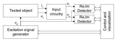
Fig. 1. Block diagram of the impedance measurement system.
