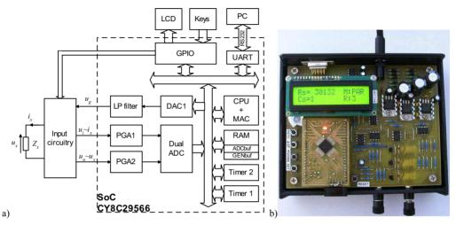
Fig. 6. Block diagram (a) and a view of prototype (b) of the particular sampling method PSoC implementation.
