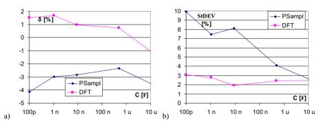
Fig. 8. Relative error (a) and relative standard deviation (b) of measurement of the reference capacitors.
