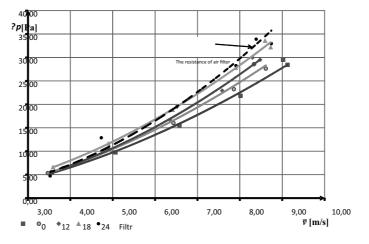
Fig. 5. The airflow resistance  $(\Delta p)$  by average airflow velocity  $(\bar{v})$ , different angle of twist tape (0, 12, 18, i 24) and air filter flow resistance
