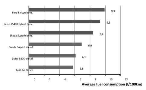
Fig. 1. Average fuel consumption by modern cars with automatic transmission[12] (test type - ADR 81)
