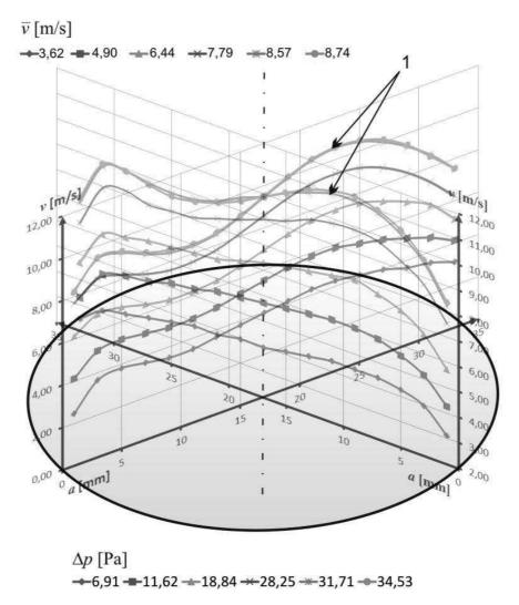
Fig. 6. The composition of velocity profiles of airflow for two mutually perpendicular planes inside the canal; 1 - the highest airflow velocity (11,2m/s)
