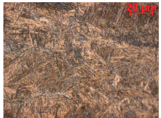
Fig. 12. Microstructure of the fusion zone magnified 1000x
