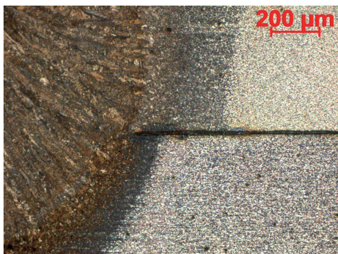
Fig. 14. Microstructure of a welded joint: the fusion zone, the HAZ and the base material; magnification: 100x
