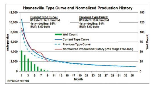
Fig. 15. Efficiency of Haynesville shale production history after fracturing (example) (Chesapeake, 2009)
