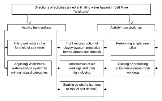
Fig. 3. Activities aimed at limiting water hazard in the Salt Mine "Wieliczka"
