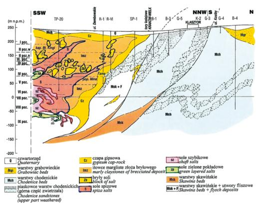
Fig. 1. Cross-section through the northern part of the mine in the transverse heading Mina area
