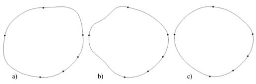
Fig. 3. Example results of a) quadratic spline b) cardinal spline c) cubic spline
