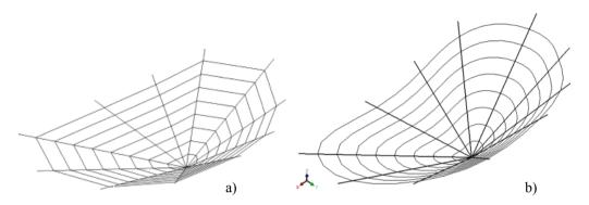
Fig. 1. Cone template constructed by (a) linear and (b) spline interpolation
