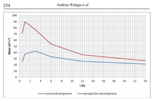
Fig. 2. The effect of watershed sealing on the size of Q<sub>max1%</sub> flows for different rainfall durations
