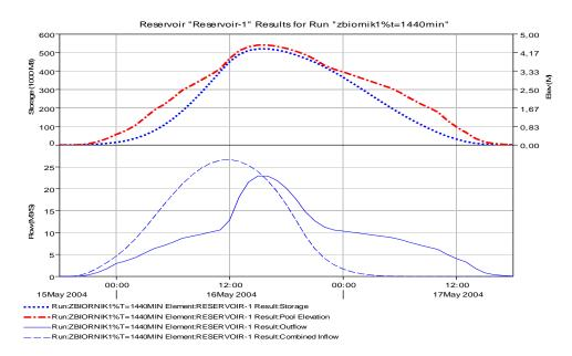
Fig. 5. Transformation of flood wave through a reservoir for the outflow of p = 1% caused by precipitation with duration of 24 h
