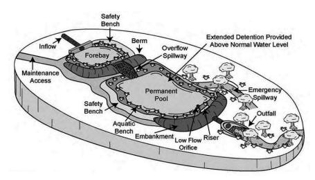
Fig. 3. Diagram of an extended retention flood detention reservoir [Wałęga 2010, after EPA 2007]
