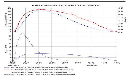
Fig. 4. Transformation of flood wave through a reservoir for the outflow of p = 1% caused by precipitation with duration of 60 min
