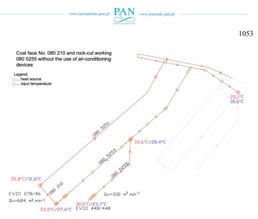
Fig. 3. Schematic diagram of calculation of expected temperatures at the workplaces of interest without the use of air-conditioning devices
