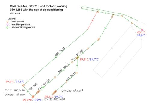
Fig. 4. Schematic diagram of calculation of expected temperatures at the workplaces of interest with the use of air-conditioning units
