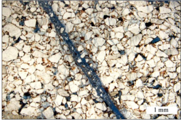
Pic. 2. Sample's cracking ( \sigma_3 = 125 MPa; \varepsilon_1 = 20\% ), enl. \times 25
