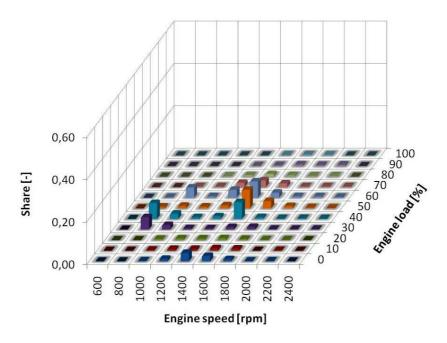
Fig. 5. Characteristics of the share of engine speeds and engine load during the test, compression ignition engine
