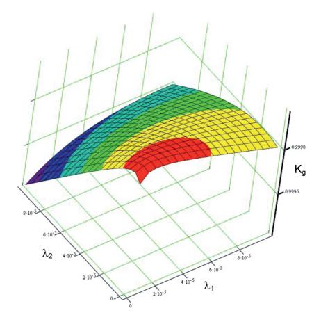
Fig. 6. Relationship between availability rate  $K_g$  as function of I type inspection coefficient  $\lambda_1$ and II type inspection coefficient  $\lambda_2$
