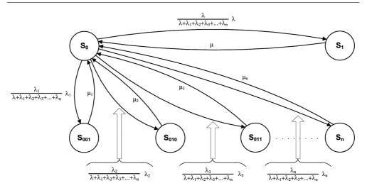
Fig. 4. Graph showing switching between usage state, repair state and I, II, III, ..., n-th type inspection state (the adjustment coefficient factored in)
