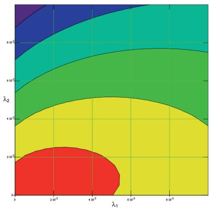
Fig. 7. Relationship between availability rate  $K_g$  as function of I type inspection coefficient  $\lambda_1$  and II type inspection coefficient  $\lambda_2$  ("top view" of contour line)
