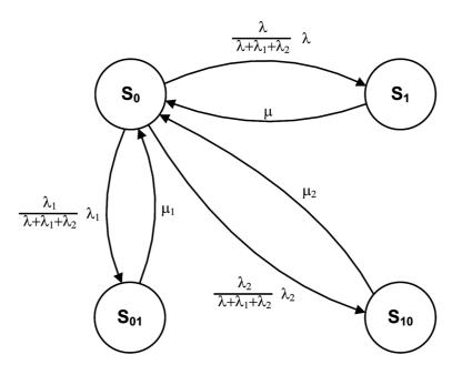
Fig. 5. Graph showing switching between usage state  $(S_0)$ , repair state  $(S_1)$ , I inspection state  $(S_{01})$  and II inspection state  $(S_{10})$  (adjustment coefficient)
