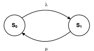
Fig. 2. Graph showing switching between usage and repair states Denotations in figures:  $\lambda$ - failure rate,  $\mu$ - repair rate
