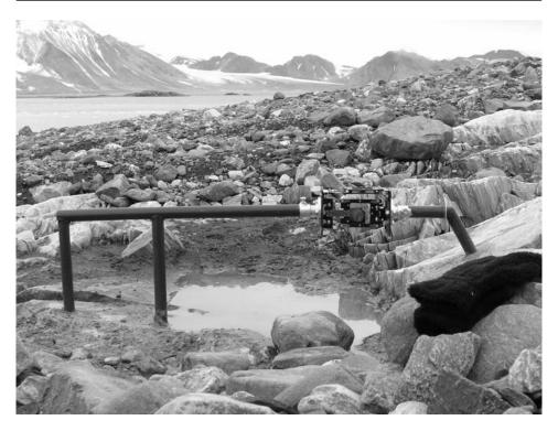
Fig. 1. The TM-71 optical-mechanical crack gauge located in front of the Hansbreen Glacier at Site 1 (Photo by T. Nýdl). The monitored fault 82°/225° crosses the outcrop beneath the instrument.
