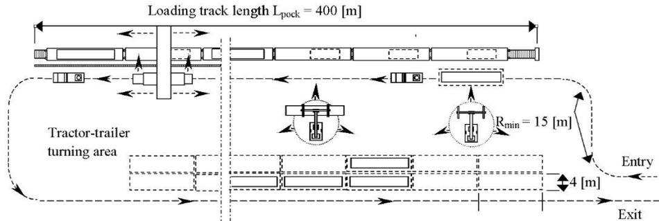
Fig. 8. Conceptual layout of an intermodal transshipment terminal for “pocket wagons” technology (a) direct transshipment realised by a gantry crane RMG; b) indirect transshipment realised by a truck mounted crane of type Reachstacker; c) direct transshipment realised by a truck mounted crane of type Reachstacker)
