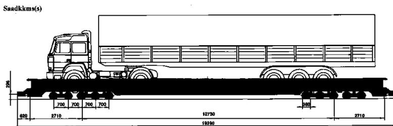
Figure 2. Low–loader platform “Ro – La” wagon, series Saadkkms
