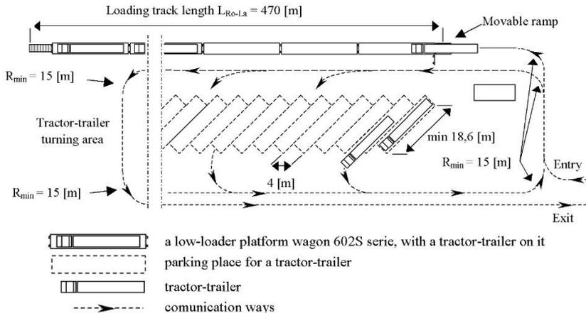
Fig. 7. Conceptual layout of an intermodal transshipment terminal for “Rollende Landstrasse” technology
