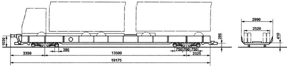
Fig. 3. Low-loader platform “Ro – La” wagon, series Saadkms
