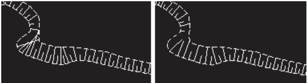
Fig. 10. Intersections of hatch lines (left), Hatch lines trimmed to the CMR (right)
