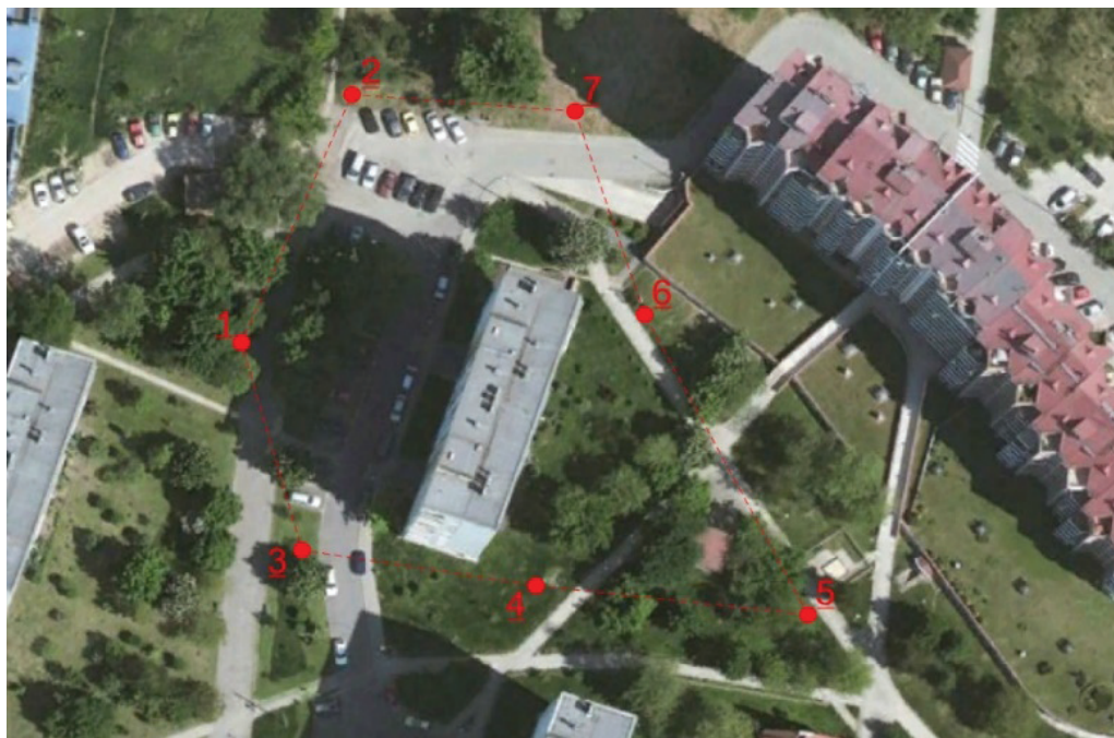
Fig. 1. The survey site with marked control network points
