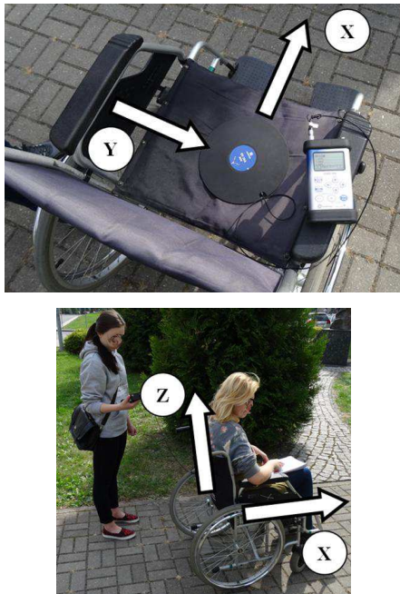
Fig. 2. Measurement instrumentation (directions of the vibration sensors' axis lines).
