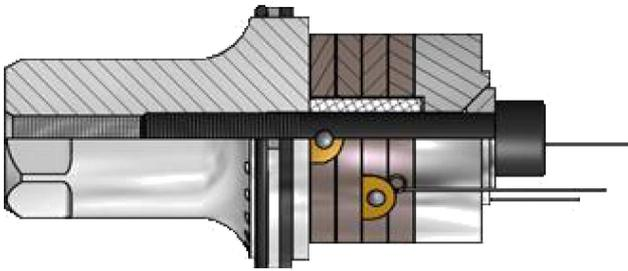
Fig. 5. Detailed geometrical model of sandwich transducer.
