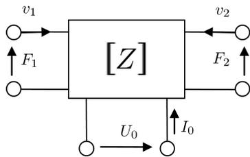
Fig. 7. Three-port network model of the piezoceramic ring.
