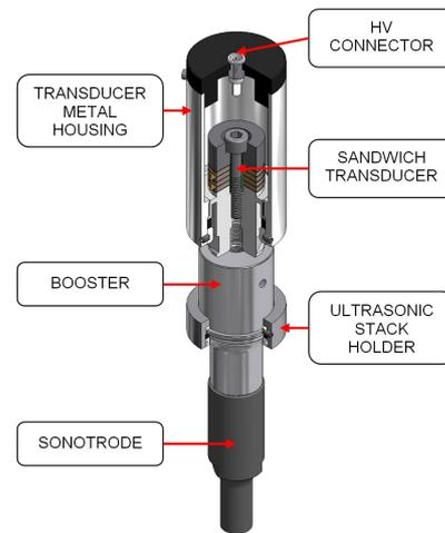
Fig. 3. Main components of the ultrasonic stack.
