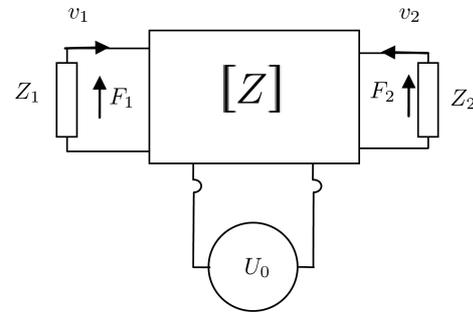
Fig. 8. Acoustically loaded model of a piezoceramic ring.
