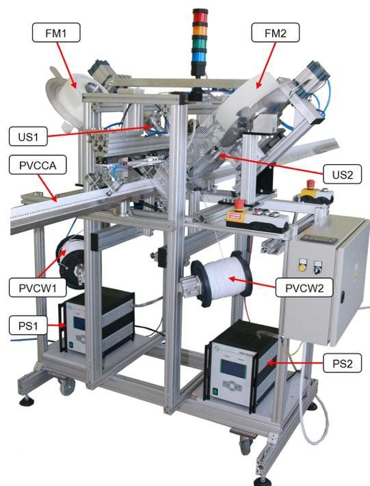
Fig. 2. Ultrasonic welding system for bonding PVC corner angles with fiberglass mesh.
