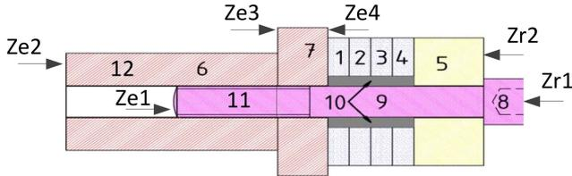
Fig. 6. Simplified geometrical model of sandwich transducer.
