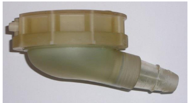
Fig. 5. Idea of the POLVAD-EXT model equipped with an additional sensor chamber (a) and the practical realization (b).
