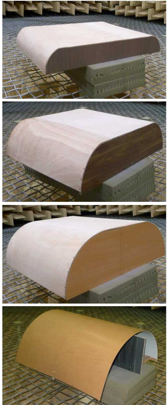
Fig. 5. Tested samples with two curved edges of radius 10 cm, 20 cm, 30 cm, 40 cm, respectively.
