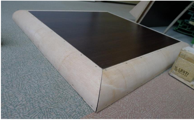
Fig. 6. The tested sample with four curved edges of radius 12 cm and total surface of dimensions 90 × 90 cm.
