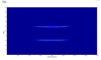
Fig. 2. The azimuth spectrum of the simulated signal [13]
