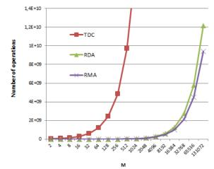
Fig. 3. Number of arithmetic operations in dependence on the number of sounding periods M
