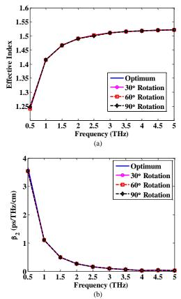
Fig. 5. (a) Effective refractive index of the reported hybrid core fiber and (b) dispersion of the reported design.
