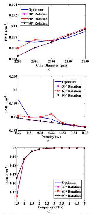
Fig. 6. EML at 1THz frequency in (a) different core diameters for 33.32% porosity, (b) for different porosity for 2450μm core diameter and (c) EML for optimum parameter of 2450μm core diameter and 33.32% porosity.
