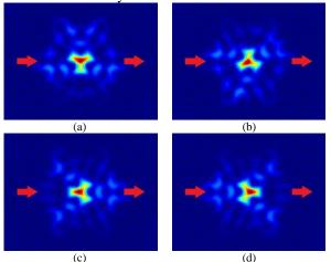
Fig. 3. Fundamental mode filed distribution for x polarization of (a) optimum design position, (b) 30° rotation, (c) 60° rotation and (d) 90° rotation.
