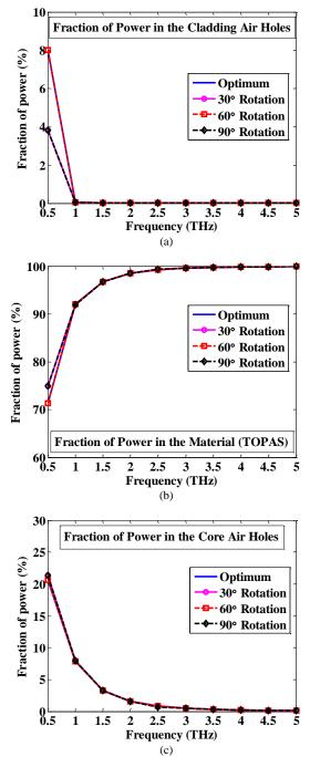
Fig. 7. Fraction of power as a function of frequency (a) in the cladding air holes, (b) in the material (TOPAS) and (c) in the core air holes.
