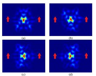
Fig. 4. Fundamental mode filed distribution for y polarization of (a) optimum design position, (b)  $30^{\circ}$  rotation, (c)  $60^{\circ}$  rotation and (d)  $90^{\circ}$  rotation.
