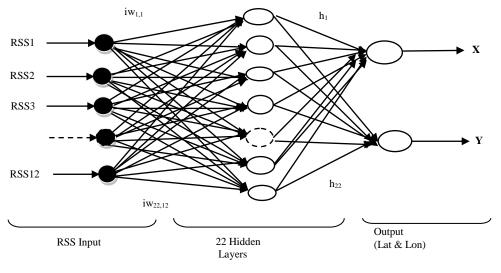
Fig. 5. Proposed Multi-Layered Perceptron architecture
