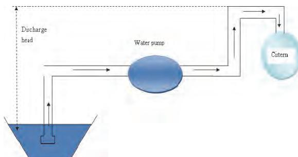
Fig. 1. Distribution of water from the reservoir into the cistern, through the water pumps; → flows;
